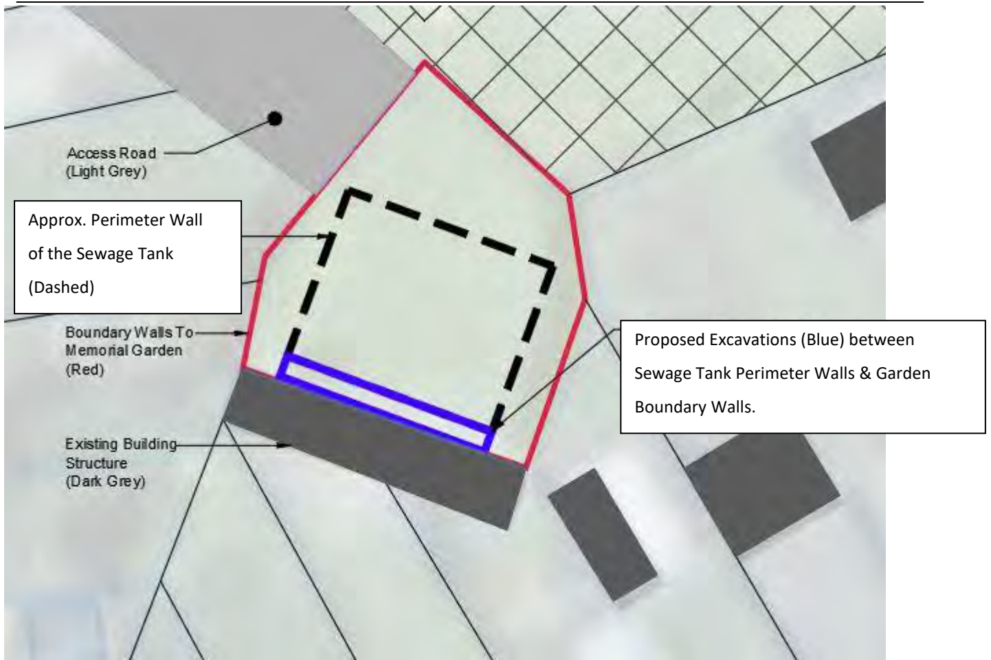
Figure 4-1 – Schematic of Sector 1, Area between Sewage Tank Perimeter Wall and Southern Boundary Walls
